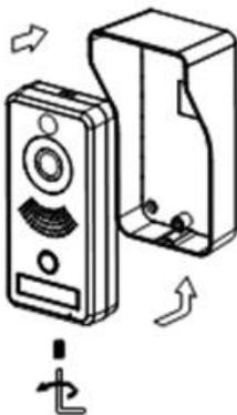
7. Fasten the camera unit rain shield with screws.
