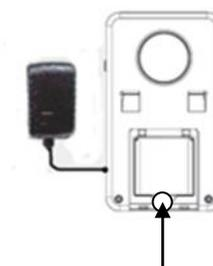
**Note that there is a magnet located in the rain shield that will trigger the alarm in the camera and on the monitor if the camera is removed when power or battery is connected.**
